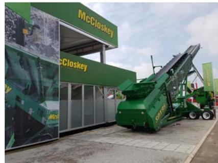
The new SDX-95 stacker desegregates and maximizes stockpile capacity using a robust, fully automated and highly flexible CAN based control system providing optimal control of material quality. It is capable of 700TPH in applications like aggregates.
