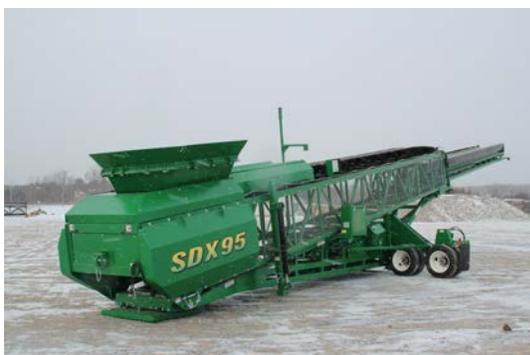
Competitively priced, the new SDX-95 is highly portable with an onboard power unit. On-site setup from truck to stockpiling can be accomplished in 15 minutes. The stacker proves to be cost effective for customers removing the need to transport a separate genset or supply mains power on site. Setup from delivery to operation can be accomplished in 15 minutes.
