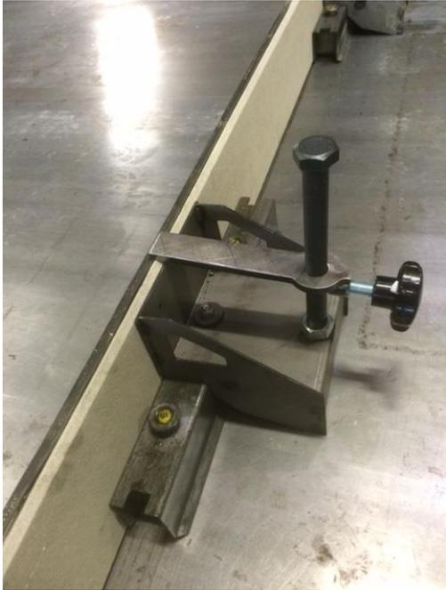
*RT U60 Pro Adapter for filigree shuttering, example with fibre concrete upstand*
