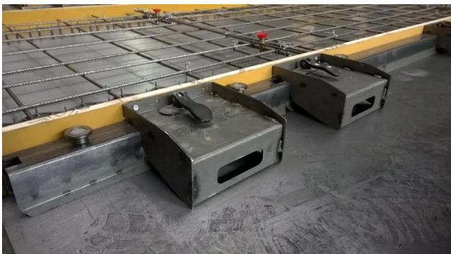
*RT U60 Pro Adapter for filigree shuttering, example with plywood*
