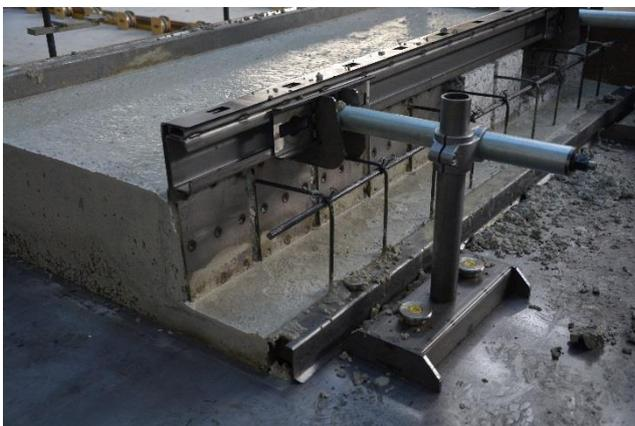
*UAR universal adapter, example of use with protruding reinforcement*
